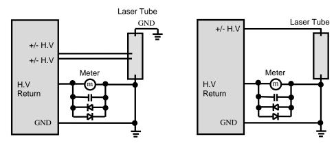
Output Configuration Wiring (FIG-4)
